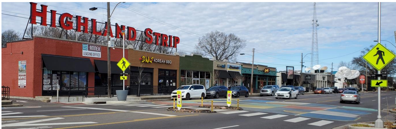
Image 2 - Memphis, TN Midblock Crossing with Continental Crosswalks, Rectangular Rapid Flashing Beacon, Pedestrian Refuge and In-Street Sign
