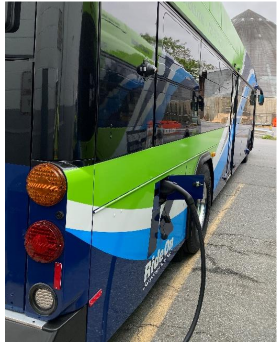
Figure 6: RideOn Bus with Plug-in Charger
