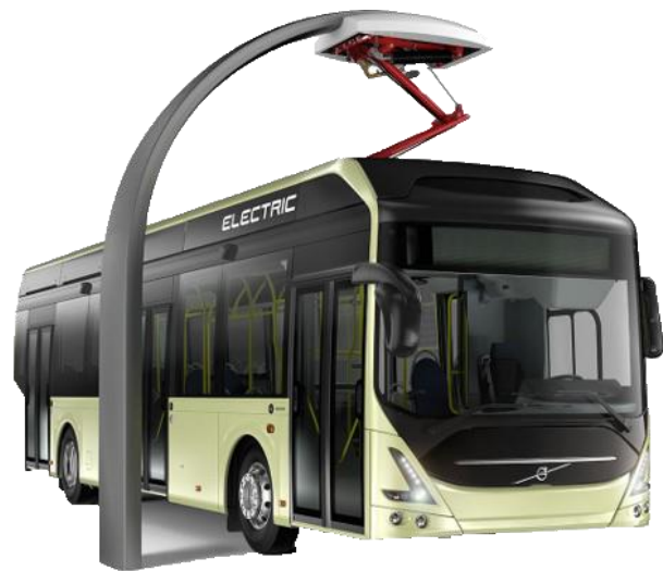
Figure 4: Bus with Pantograph Charger
