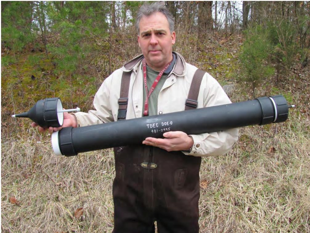
**Figure 3: Photo of Sediment Trap**
