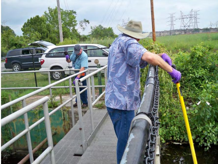
**Figure 2: Storm water sample collection at P-1 Pond Weir**
