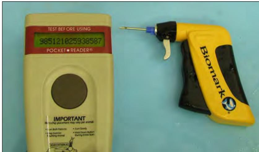
**Figure 5: Passive Integrated Transponder (PIT) tag equipment for identification of fish recaptures.**
