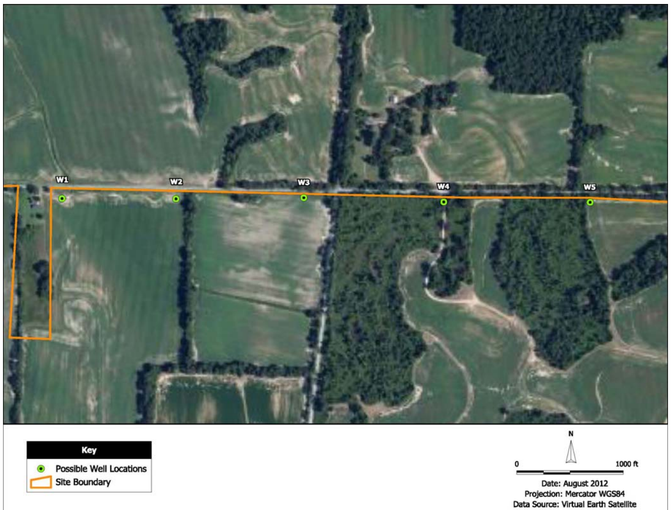
Figure 5. Possible well locations for 8 mgd well field.
