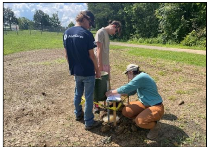
Below: Infiltration testing at Gibbs Ruritan Park
