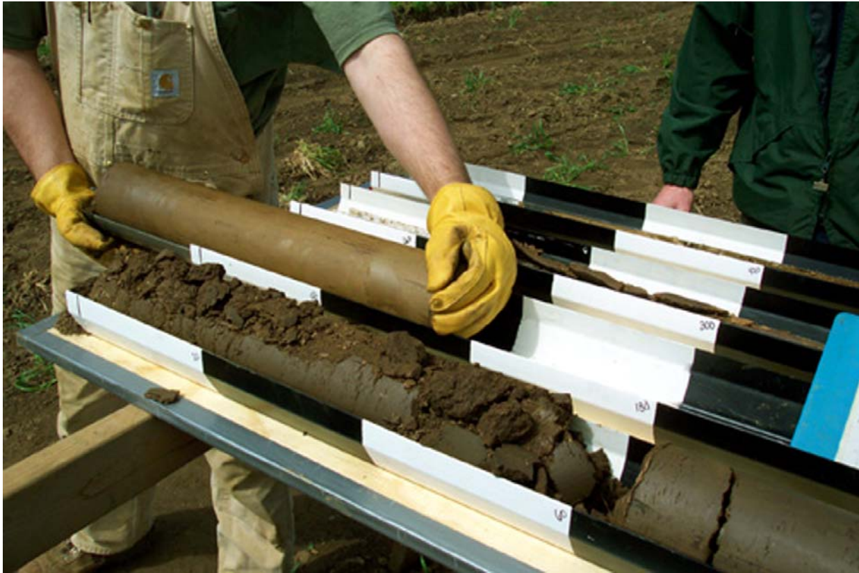
FIGURE 3. Four-inch core removed from split spoon and placed into the ARL table designed to facilitate the field description, photo-documentation, and sampling of core sections.
