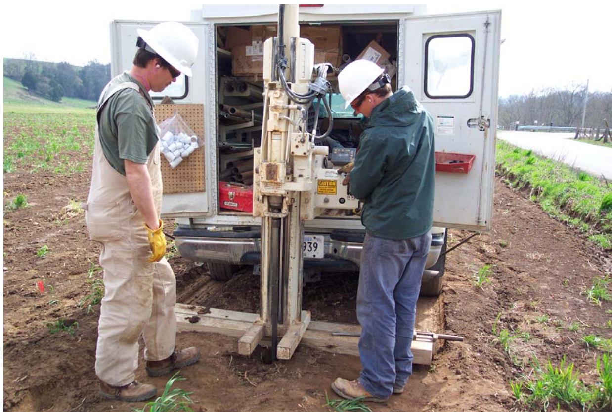
FIGURE 2. MACTEC operation of Geoprobe 5400® during the project.
