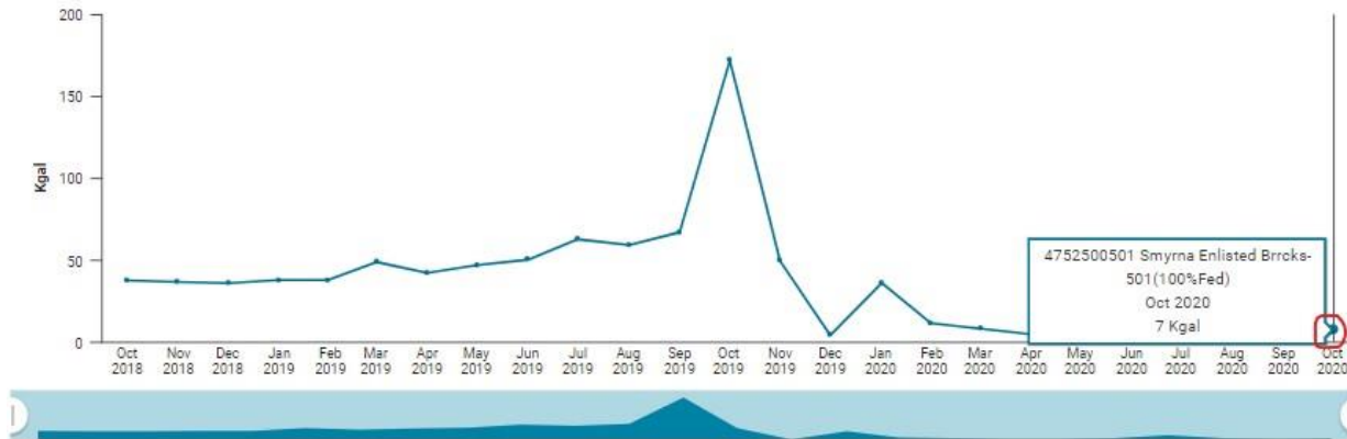
[A.3] Figure 6.3.1c – Department of Military October 2020 Water Usage after Water Leak Repair (UDM Dashboard)
