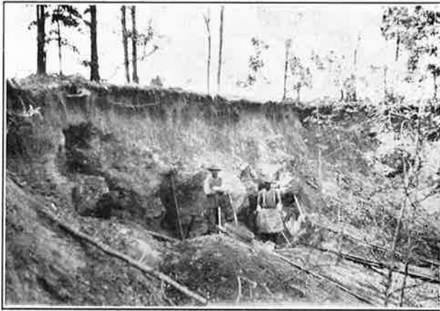
(A) Deposit of brown iron ore near Cumberland furnace, Dickson County, being mined by hand, hand cobbled, and dry screened.
