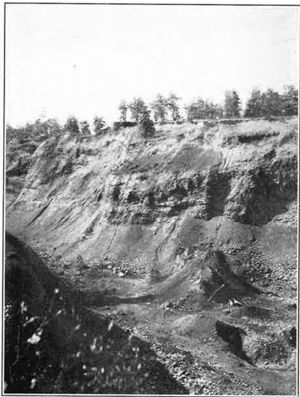
(A) Deep cut in Napier brown iron ore mine, Lewis County, showing disintegrated chert in wall.
