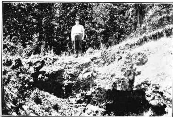
(A) Face of brown iron ore ledge in Swamp Bank of La Grange property, Stribling, Stewart County. Right end of ledge at hammer handle shows a band of chert.
