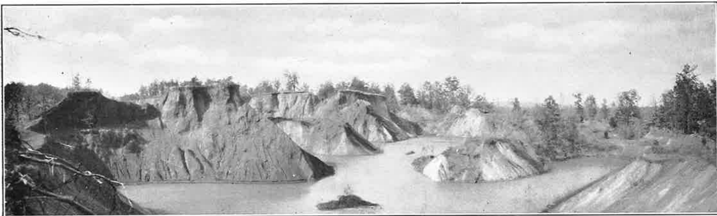
(A) Nunnely brown iron ore mines, Hickman County, October, 1921. Bank at left is red loam at top with talus below covering "white-horse" clay. Farther to the right "white-horse" clay is shown.
