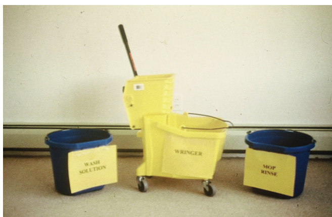
FIGURE 14.4 Three-bucket cleaning system.
