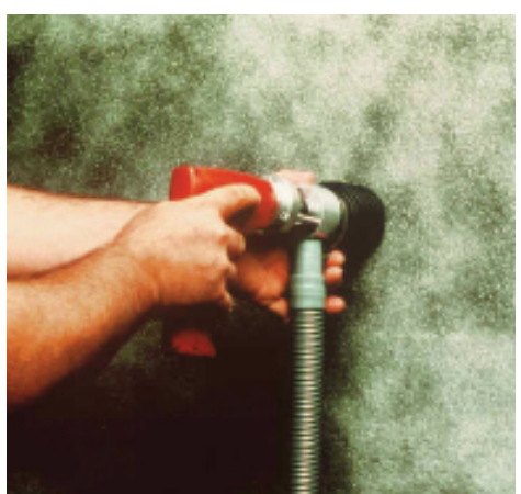
FIGURE 12.19 Needle Gun with HEPA Exhaust Ventilation.
