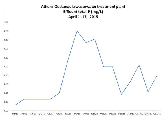
To monitor conditions, daily in-house testing was performed using a spectrophotometer for the rest of the study period. Data were compiled and reviewed at least weekly. Samples were collected in the following locations and testing for soluble phosphorus, ortho-P:
