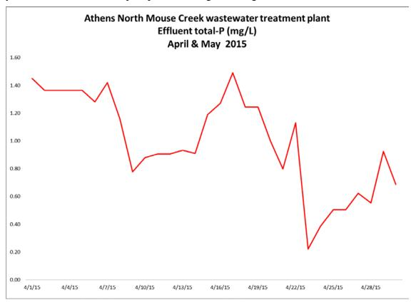
*Phosphorus*. In advance of the consultant's first visit, plant staff installed a pump in a thickened sludge holding tank and pumped a small amount back into the plant's headworks daily. As with Oostanaula, the early results were encouraging. By late-April effluent total-P was the lowest that plant staff ever recalled seeing. For almost a week, the concentration remained below 0.5 mg/L.
