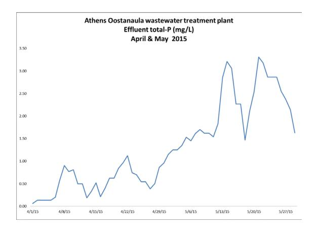
In-house testing documents that the fermentation tank is effectively releasing ortho-P. And, at times, too much ortho-P is released. Conditions are suitable for aerobic ortho-P uptake: high dissolved oxygen (DO) and pH of 7.0 or higher. It appears that phosphorus is being re-released in the plant but plant staff has not been able to locate where the release is occurring. Monitoring of the ortho-P concentration in the RAS (return activated sludge) is performed to see if the over-
