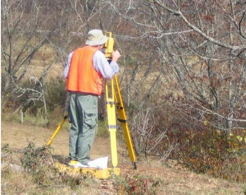
Figure 2-2. Using a total station to survey a stream.
