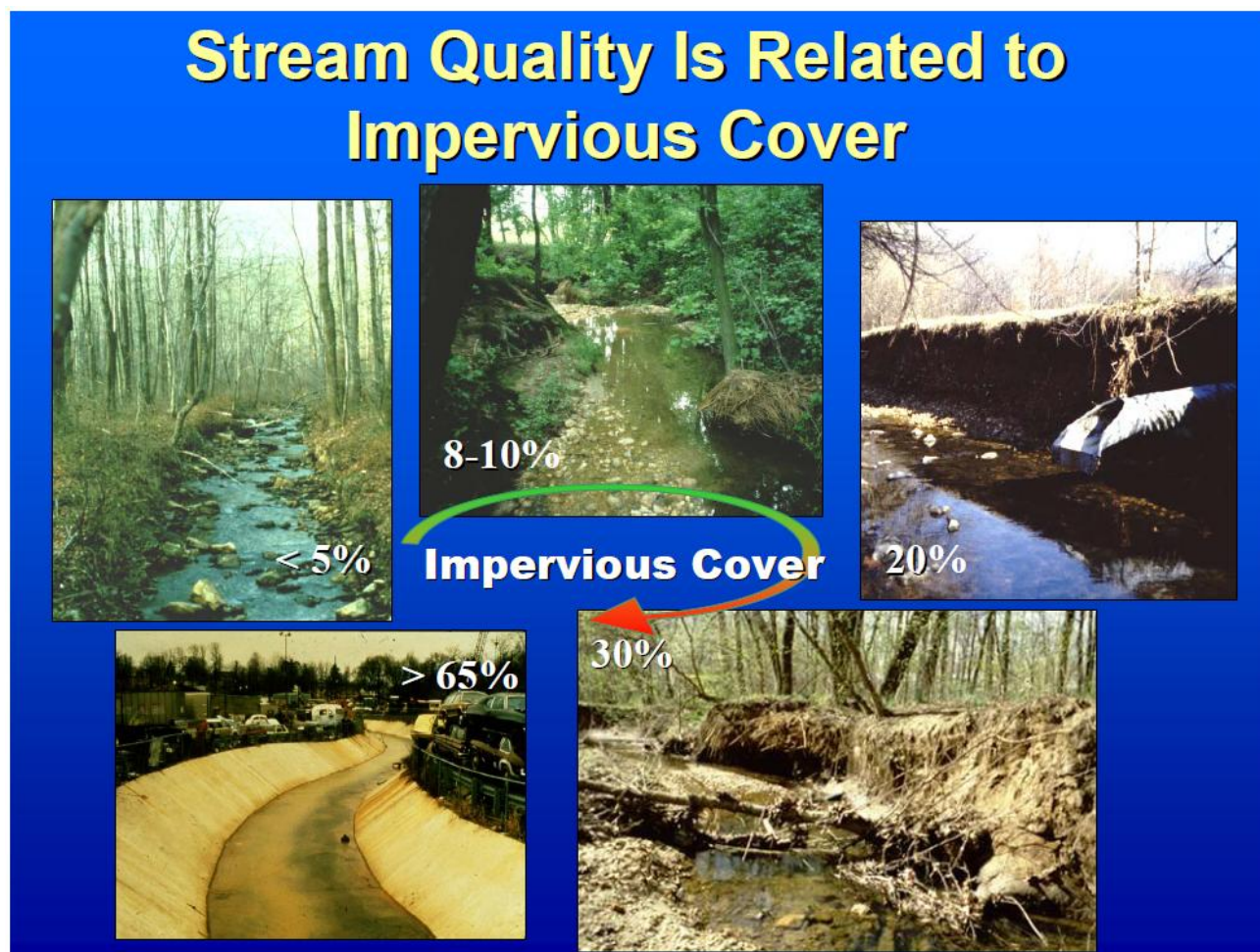
Figure 21. Effects of % impervious cover in the upstream watershed.
