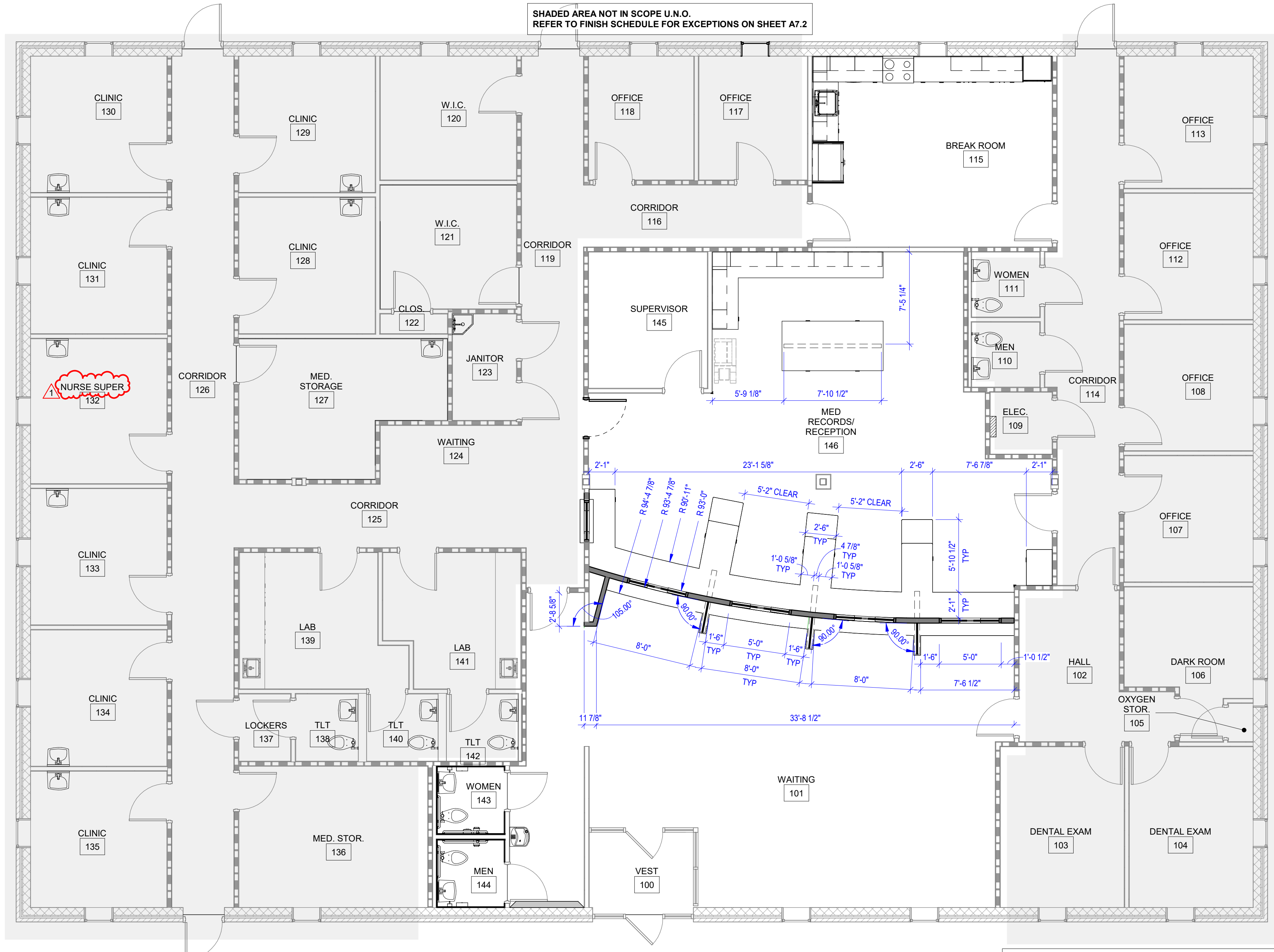
D2 FLOOR PLAN - DIMENSIONED 3/16" = 1'-0"
