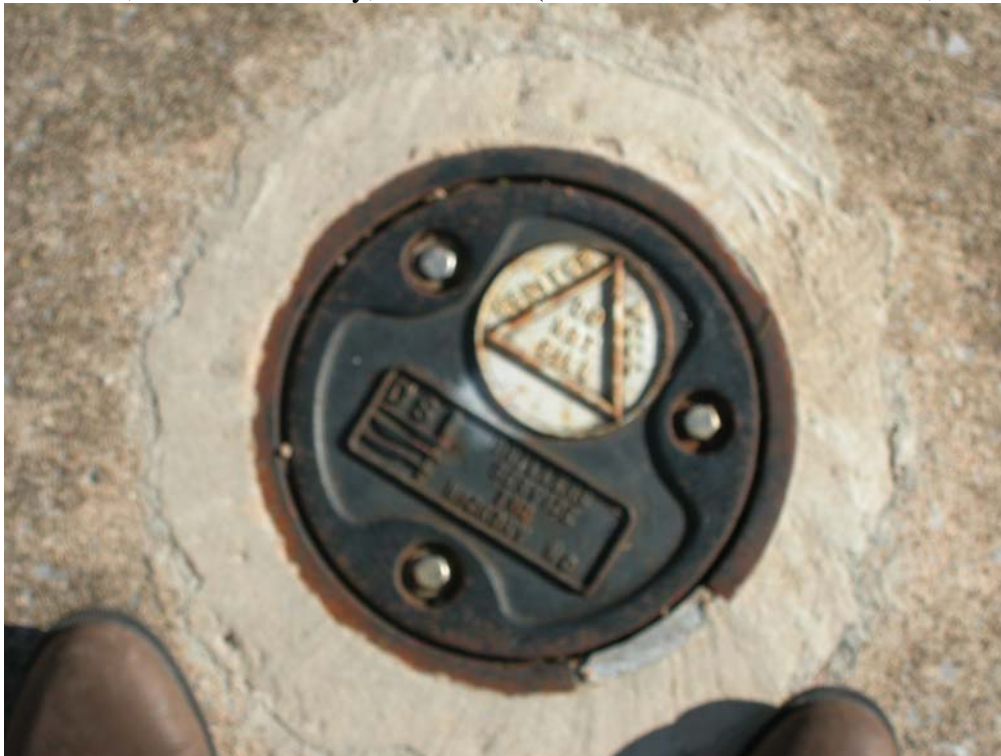
FIGURE 5 - Photo of monitoring well cover. Nashville, Davidson County, Tennessee (Photo credit: David Borowski, TDH, 11/19/03)
