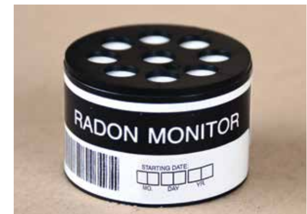
PHOTO: Testing to see if a radon mitigation system should be included in your restoration plan is inexpensive and easy. Radon test kits are available from home improvement stores.
