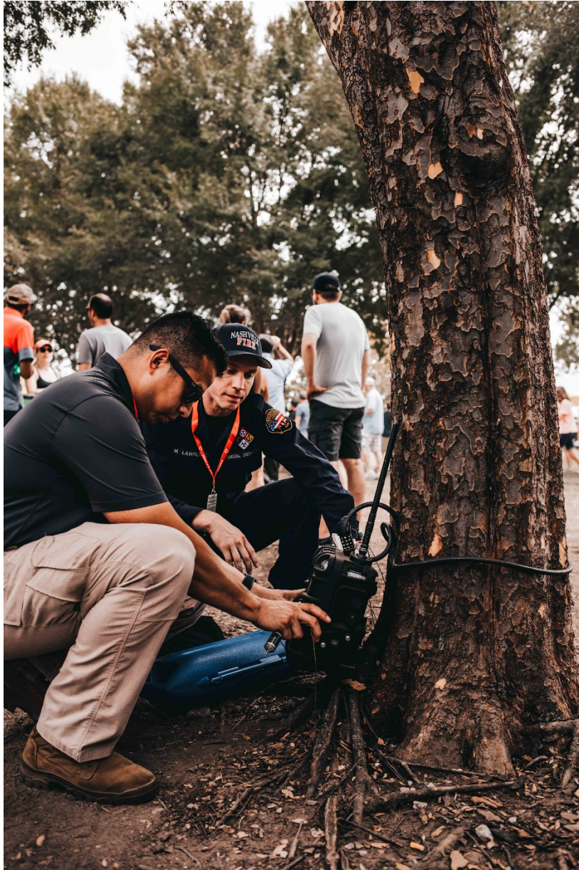
Sgt. Christopher Barriere, a member of the 45th Civil Support Team, and Michael Lawrence, a member of the Nashville Fire Department Special Operations Unit, set up air monitoring systems around the Music City Grand Prix, August 7, in Nashville. These air sensors monitor for radiation, chemicals, carbon monoxide and explosives in areas of heavy foot traffic during the event. (Photo by 1st Lt. Sarah Kohrt)
