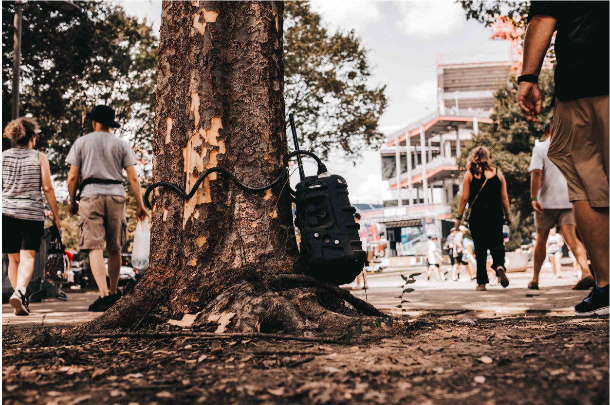
An AreaRAE air monitoring system is stationed against a tree, outside Nissan Stadium, August 7, during the Music City Grand Prix. The 45th Civil Support Team sets up these sensors to monitor for radiation, chemicals, carbon monoxide and explosives in areas of heavy foot traffic during the event. (Photo by 1st Lt. Sarah Kohrt)
