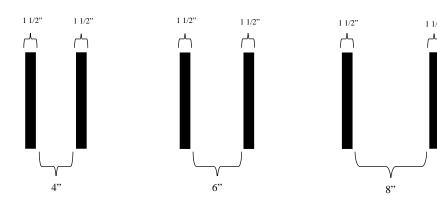
Contrast striping, 4-inch with 1-1/2 inch black border Contrast striping, 6-inch with 1-1/2 inch black border Contrast striping, 8-inch with 1-1/2 inch black border
