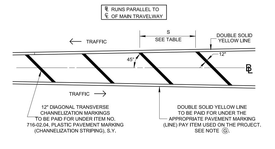
FOR MEDIAN WIDTH LESS THAN 6' NO DIAGONAL MARKING WILL BE REQUIRED (MEASURED OUTSIDE OF BOUNDARY LINES).
