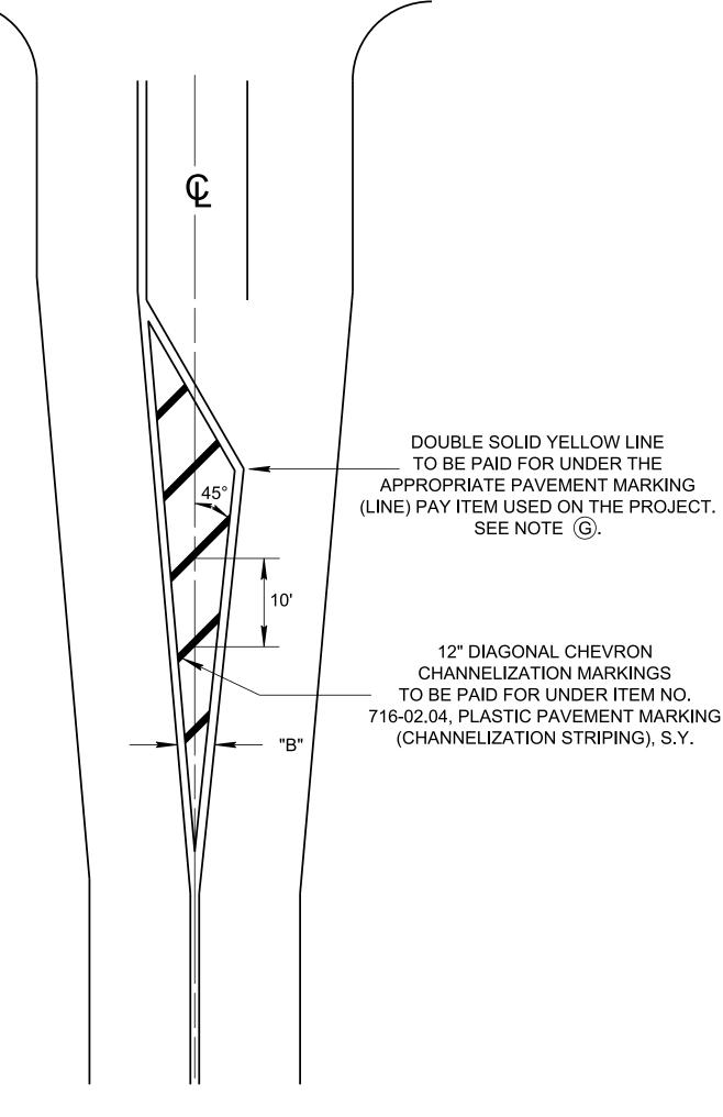
LEFT TURN CHANNELIZATION ISLAND WHEN WIDTH "B" IS LESS THAN 6' (MEASURED PERPENDICULAR TO THE G) NO DIAGONAL MARKING WILL BE REQUIRED.
