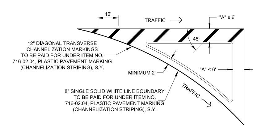
WHEN DISTANCE "A" IS LESS THAN 6', NO DIAGONAL MARKING WILL BE REQUIRED (MEASURED FACE OF CURB TO OUTSIDE OF BOUNDARY LINE).
