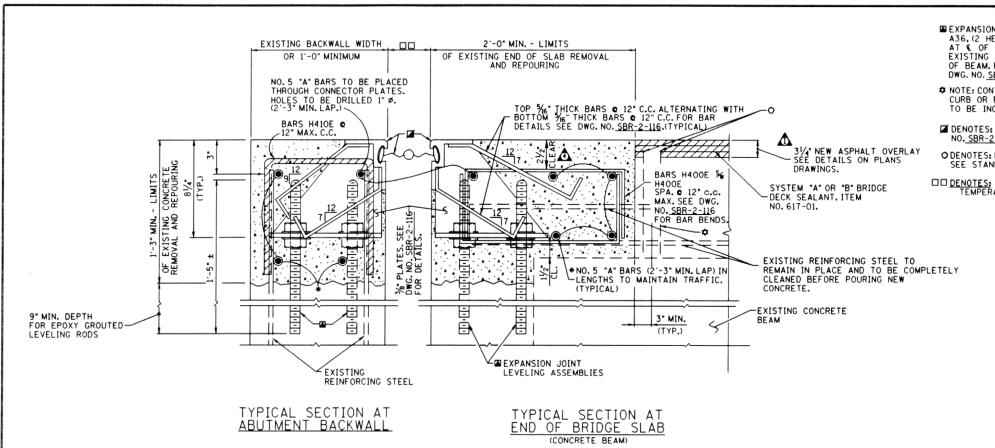
■EXPANSION JOINT LEVELING ASSEMBLIES - TWO (2) 1/8" Ø THREADED RODS, ASTM A36. (2 HEX NUTS AND 2 - 3½" X 3½" X 3½" X 3½" SOUARE WASHERS PER BOLT), LOCATED AT € OF EACH BEAM. DRILL AND EPOXY GROUT THREADED RODS 9" INTO EXISTING ABUTMENT BACKWALL AND EXISTING END DIAPHRAGM, OR END OF BEAM. FOR OTHER EXPANSION JOINT LEVELING ASSEMBLY DETAILS SEE DWG. NO. SBR-2-116.
