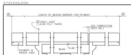
MEDIAN & BENT ELEVATION OF MEDIAN BARRIER WITH CONSTRUCTION JOINT
