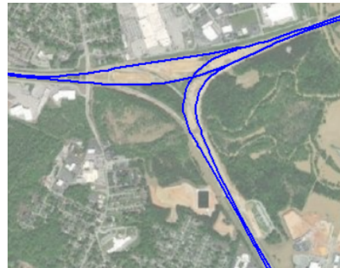
Figure 1. Example of Segments Missing at a System Interchange (NPMRDS data in blue)
