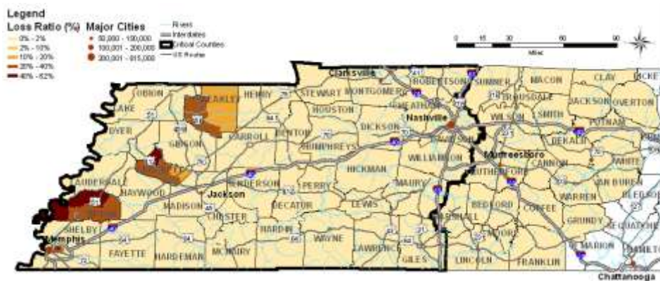
Figure 2 – NMSZ Event Loss Ratio (% of Total Building Assets) for State of Tennessee [Source: MAE Center, 2008]
