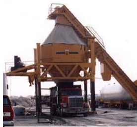
Portable Surge Silo
