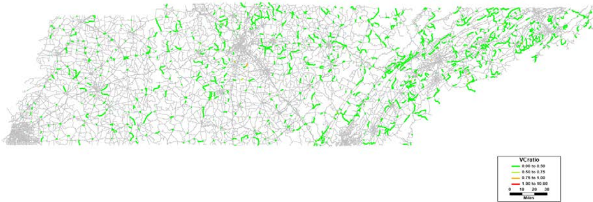
Figure 131: Volume to Capacity Ratio for Non-Interstate Urban Roads with Speed Limit less than 40 mph (2040)
