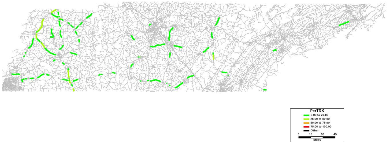
Figure 48: Percentage of Trucks for Non-Interstate Rural Roads with Speed Limit greater than or equal to 60 mph (2010)
