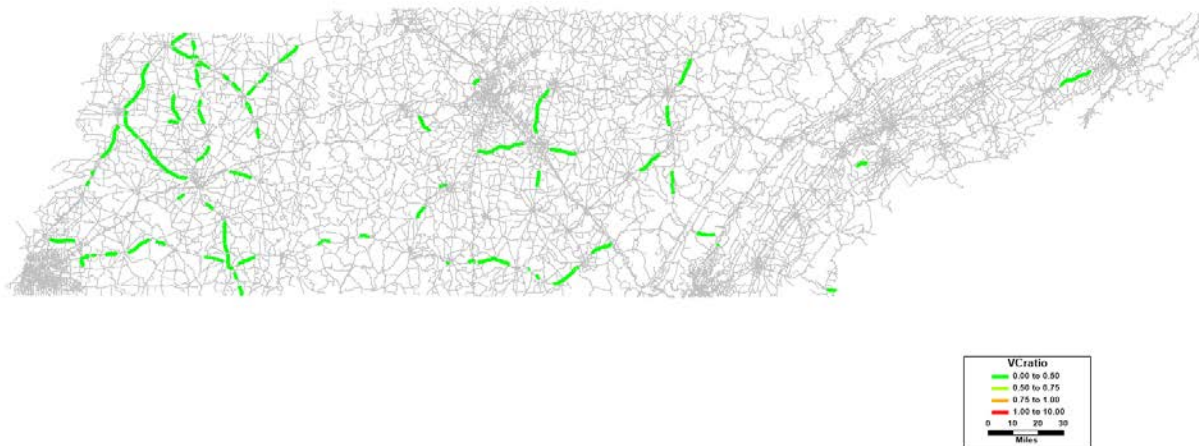
Figure 50: Volume to Capacity Ratio for Non-Interstate Rural Roads with Speed Limit greater than or equal to 60 mph (2010)
