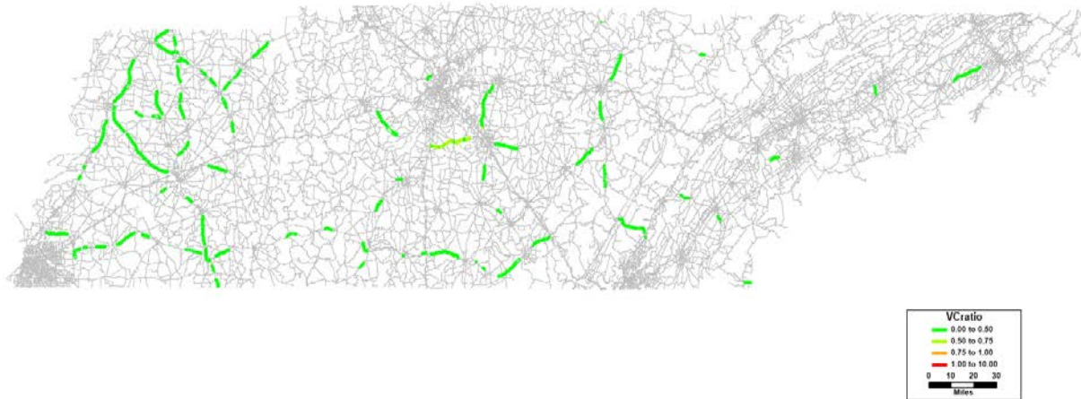
Figure 106: Volume to Capacity Ratio for Non-Interstate Rural Roads with Speed Limit greater than or equal to 60 mph (2040)
