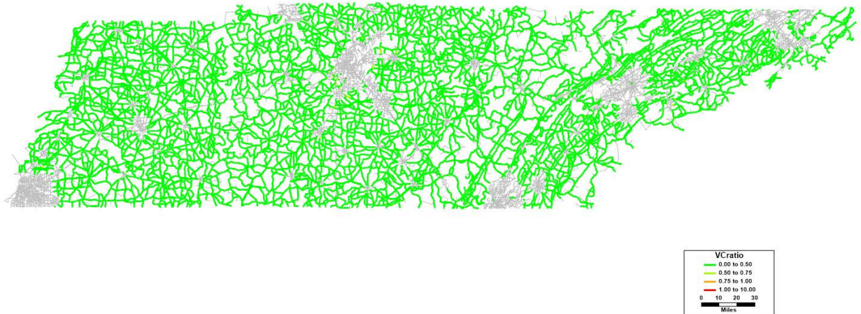
Figure 55: Volume to Capacity Ratio for Non-Interstate Rural Roads with Speed Limit greater than or equal to 40 and less than 60 mph (2010)
