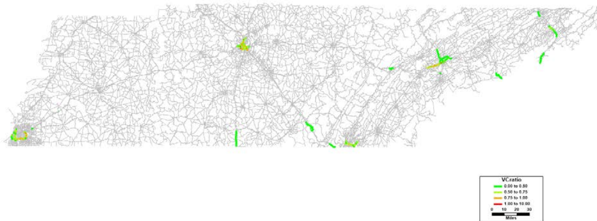
Figure 45: Volume to Capacity Ratio for Interstates with Speed Limit less than 65 mph (2010)
