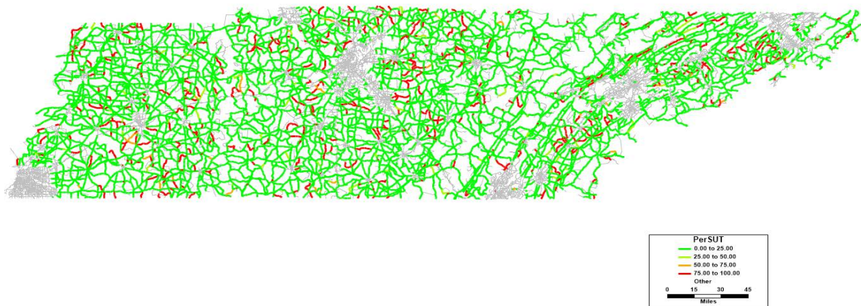
Figure 52: Percentage of SUTs for Non-Interstate Rural Roads with Speed Limit greater than or equal to 40 and less than 60 mph (2010)
