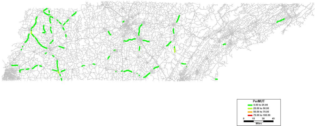
Figure 46: Percentage of MUTs for Non-Interstate Rural Roads with Speed Limit greater than or equal to 60 mph (2010)
