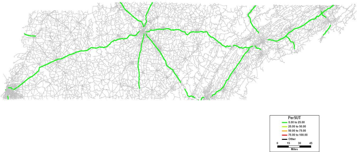
Figure 37: Percentage of SUTs for Interstates with Speed Limit greater than or equal to 65 mph (2010)
