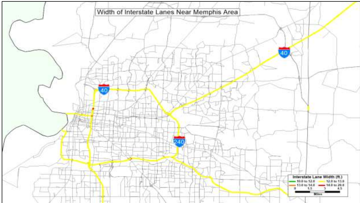
Figure 2.17. Memphis Interstate Lane Width
