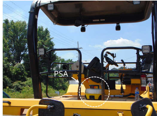
(b) PSA on a roller compactor
