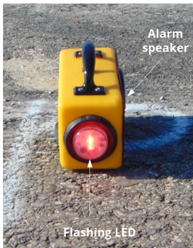
(b) Portable Alarm Case (PAC) showing LED and position of the alarm speaker
