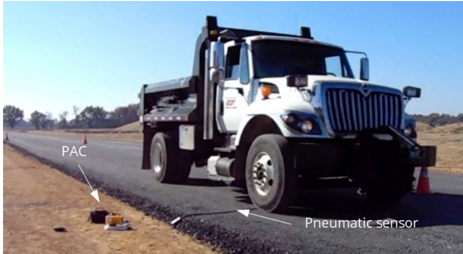
Figure 4-19. Test vehicle running over the pneumatic sensor
