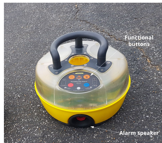
(b) Portable Site Alarm showing layout of functional buttons and alarm speaker
