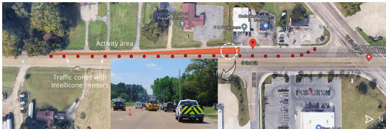
Figure 4-31. Project 4: Arrangement of Intellicone components
