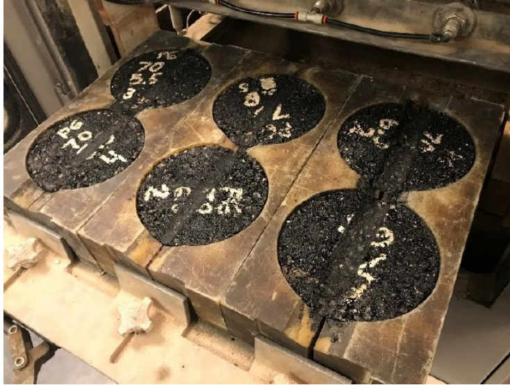
Figure A-8. Test specimens after 8000 cycles.
