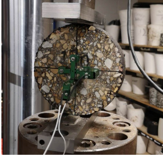
Figure A-6. Setup for Superpave IDT tests.
