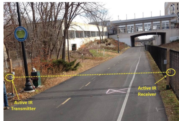
Figure 13: Active infrared counter installation at a test site. Source: Tony Hull, Toole Design Group (Ryus et al., 2014b).
