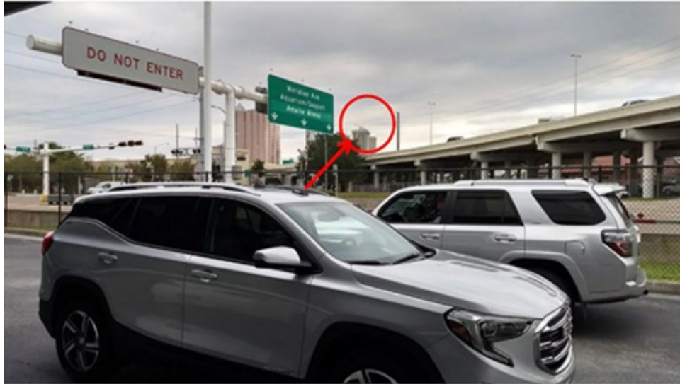
Figure 5-1 The position of the vehicle and OBU antenna on that as well as the line of sight to the HamWAN radio antenna
