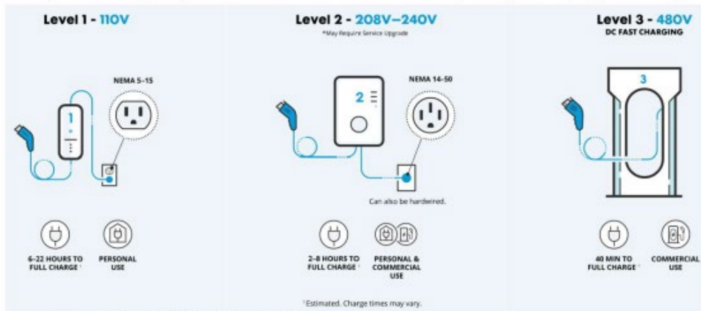
Figure 3: Levels of Electric Vehicle Charging. (Source: ConEdison)
