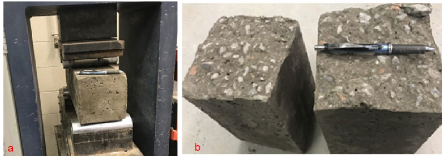
(a) Third Point Loading (b) Example of Failure Section Figure 3.2.3 Flexural Test Setup
