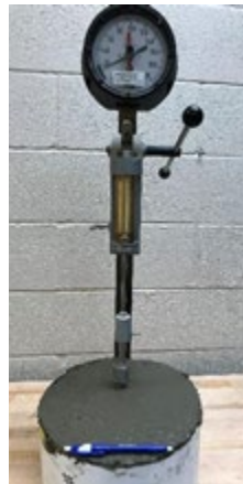
Figure 3.2.2 Test Setup for Time of Setting of RCA Concrete
