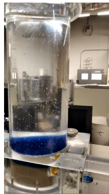
Figure 4-17. AVA test of fresh Class A concrete (Region 1)
