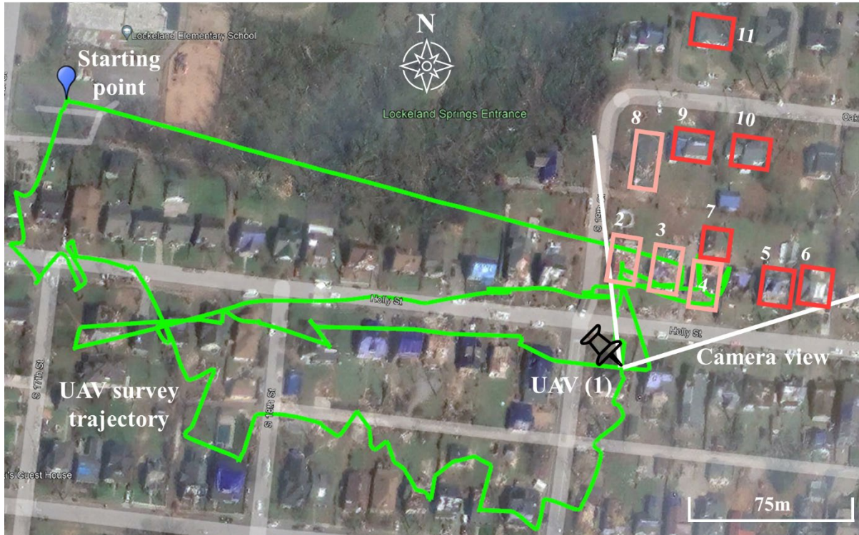
Figure 4-7 Drone Survey Trajectory and Overlaid Detected Damaged Buildings.
