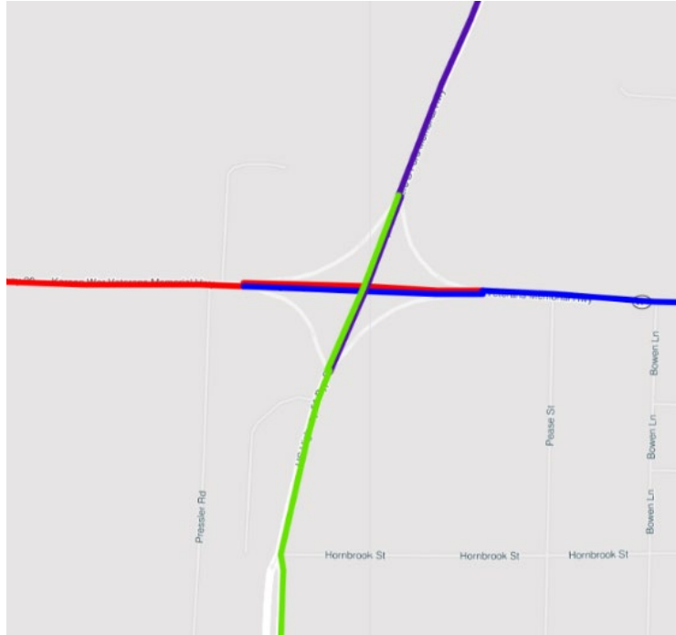
Figure 3.3 (a) A crossroad intersection at TN-104 and US-51 BYP. Four different pairs of TMC segments did not have a singular end GPS coordinate but had a match for road and intersection names.
