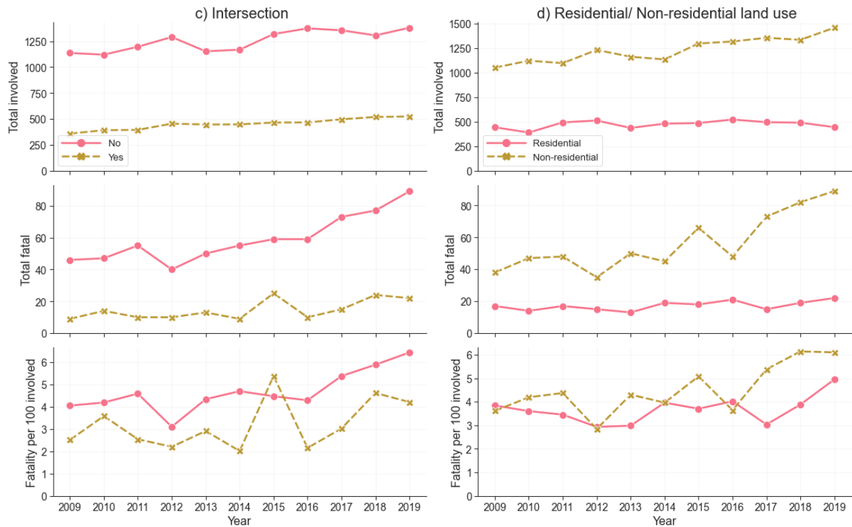
Figure 4.9 Pedestrian Crash Trends a) Posted Speed Limit, b) number of lanes, c) intersection and non-intersection locations d) Residential and non-residential land uses
