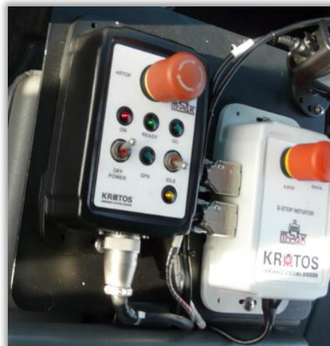
Figure 11 - Leader Vehicle Internal A-Stop and E-Stop Buttons
