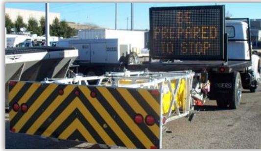
Figure 2 - TMA used in TDOT's Protect-the-Queue Program
