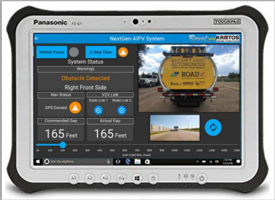
Figure 9 - Graphic User Interface (GUI) device located on Leader Vehicle
