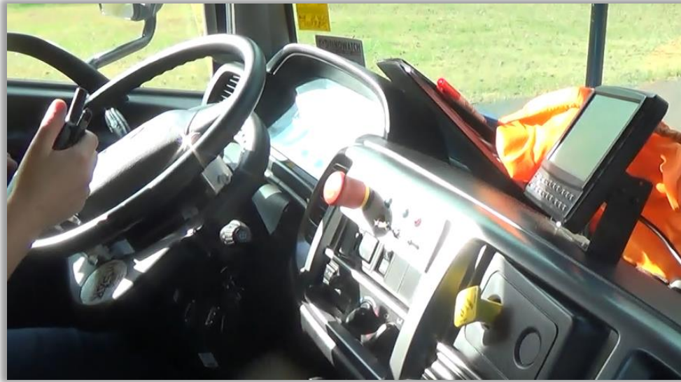
Figure 13 - AIPV Internal E-Stop Button
