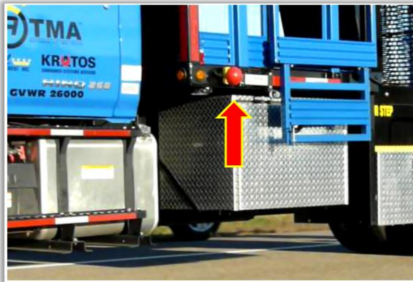
Figure 12 - AIPV External E-Stop Button
