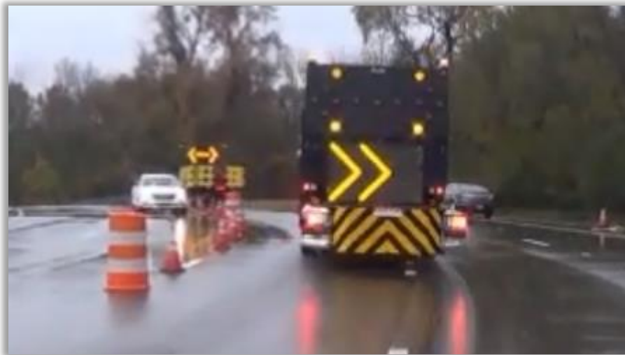
Figure 53 – ATMA System during Headlights Test
