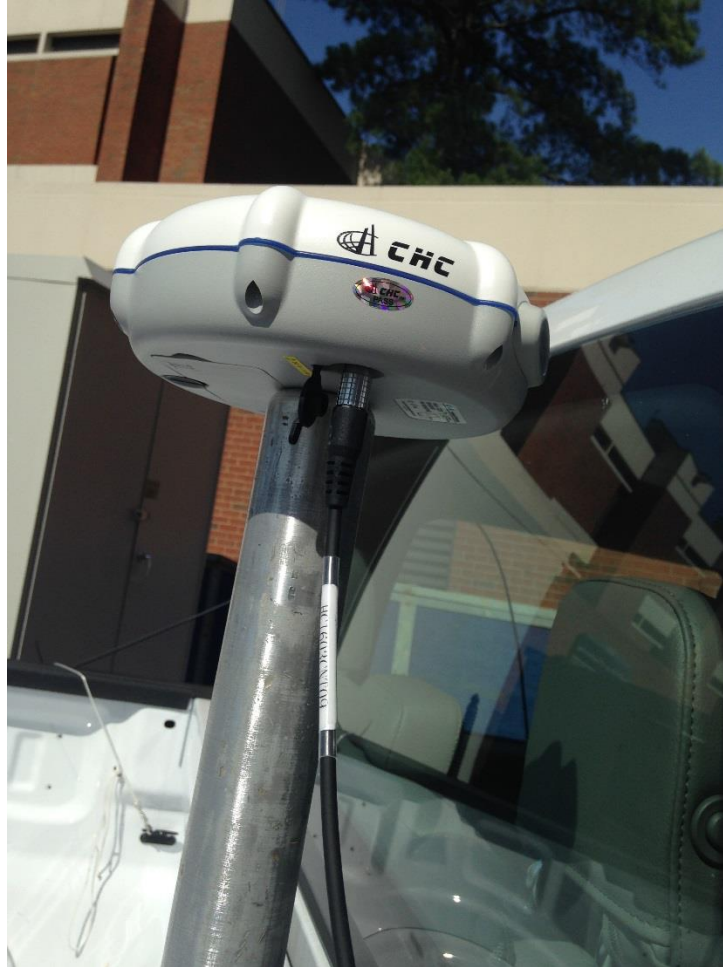
Figure 8: GPS mounted on the back of the truck.
