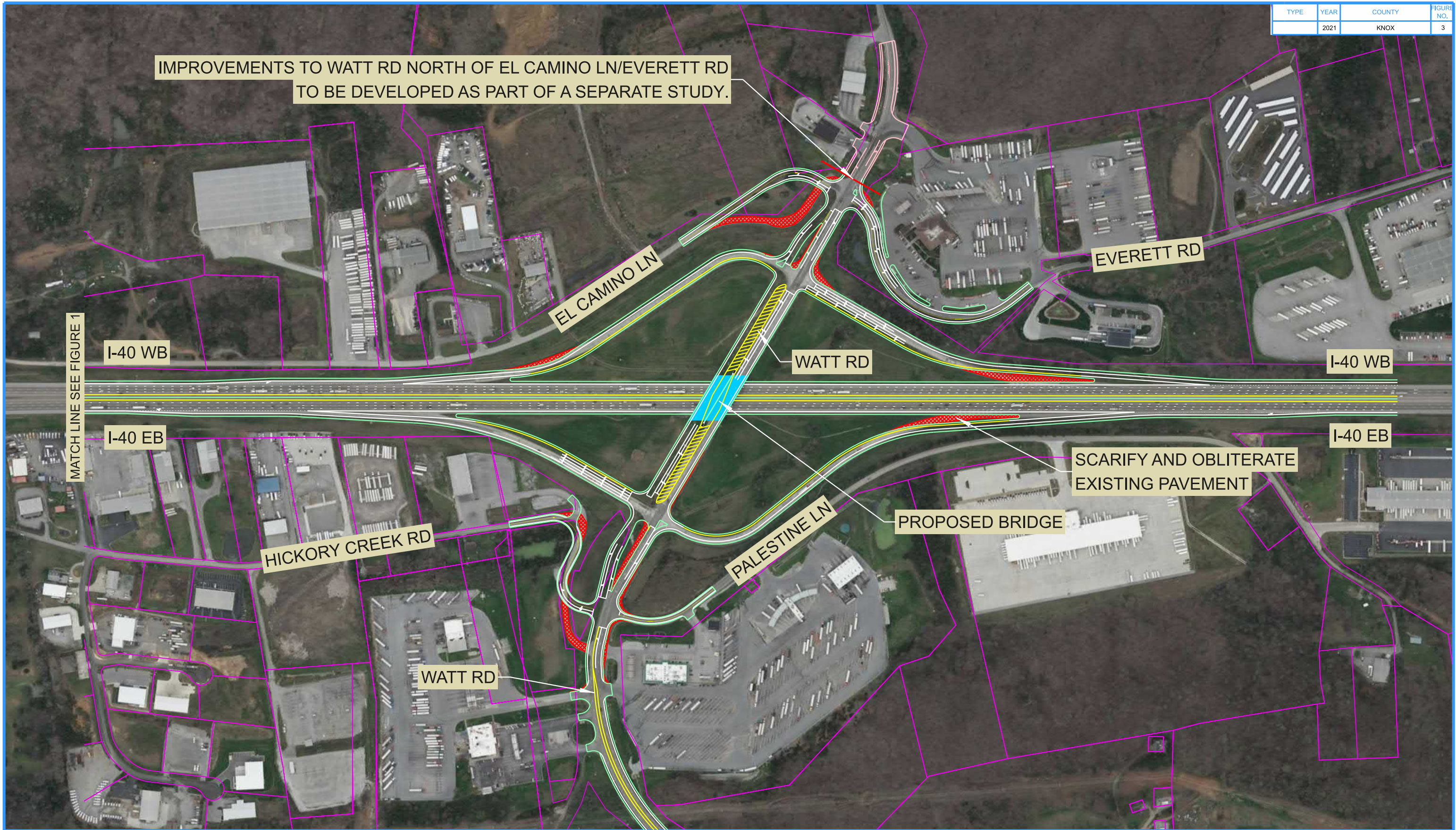
FIGURE 3 BUILD ALTERNATIVE #2 DIAMOND INTERCHANGE WITH IMPROVEMENTS
