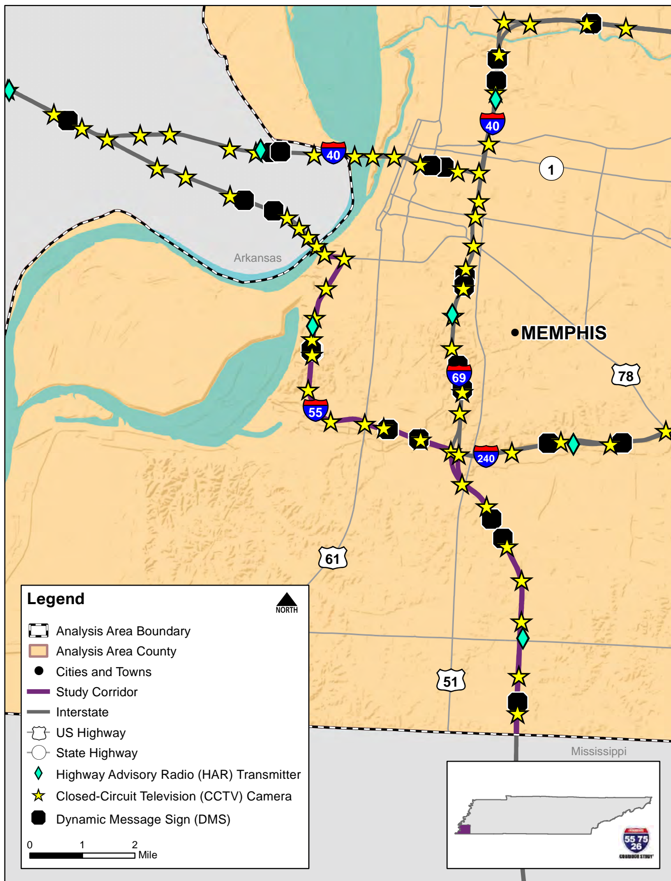
Figure 5-3. Intelligent Transportation System Components — I-55
