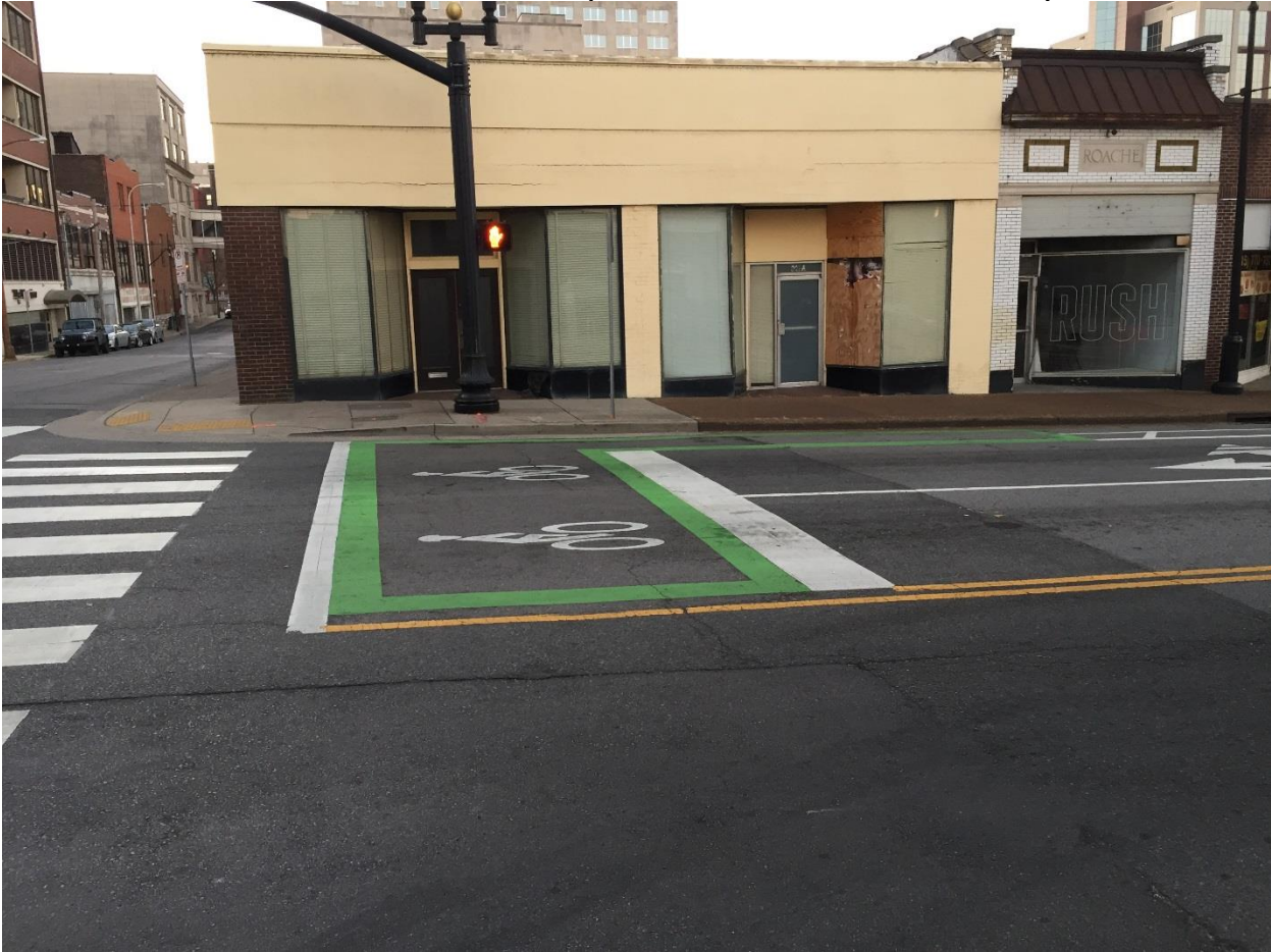
EXHIBIT 6-10: BICYCLE BOX (WITH GREEN PAVEMENT MARKINGS)
