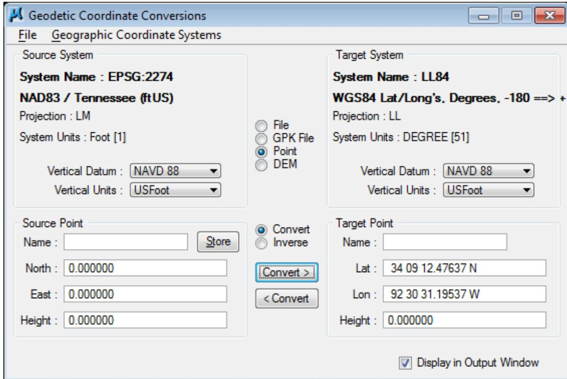
The Source System should be set automatically from the DGN file coordinate system settings and the Target System may already be set as well. If your systems are not set as shown above, go to the drop down option **Geographic Coordinate Systems> Select**.
