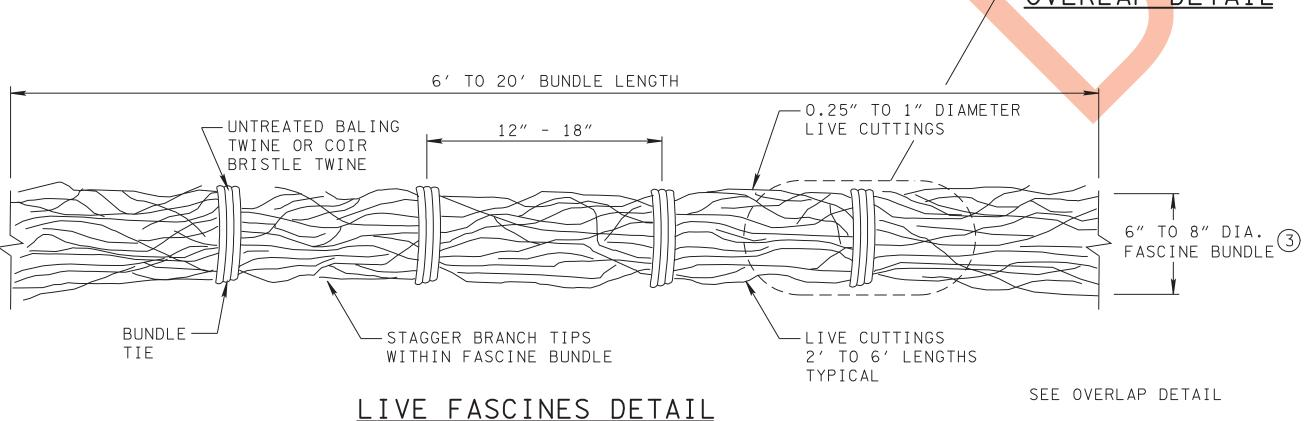
NOTE (3): FINAL DIAMETER WHEN FIRMLY COMPRESSED AND TIED
