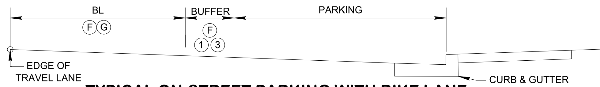
TYPICAL ON-STREET PARKING WITH BIKE LANE
