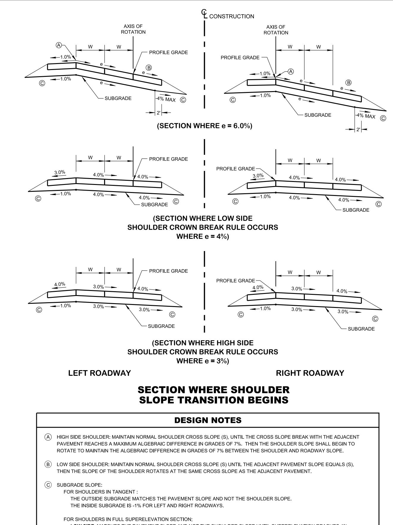
LOW SIDE MATCHES THE PAVEMENT SLOPE AND NOT THE SHOULDER SLOPE UNTIL SUPERELEVATION REACHES 4%. WHEN THE SUPERELEVATION IS GREATER THAN 4% THE SUBGRADE WILL HAVE A BREAK IN SUBGRADE 2' BACK UNDER THE SHOULDER AND THE GRADE RUNNING OUT WILL MAINTAIN A 4% SLOPE. SEE SECTION D-D FOR DETAILS. HIGH SIDE SHOULDER AND ADJACENT PAVEMENT SUBGRADE CHANGE MUST NOT EXCEED AN ALGEBRAIC DIFFERENCE IN GRADES OF 7%.
